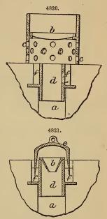
fuel the firing holes with their cones are kept closed by the cap or cover e, which is maintained air-tight, or nearly so, by the joint f. C. E. E. Muller has effected an arrangement of kiln for carrying out a mode of heating
